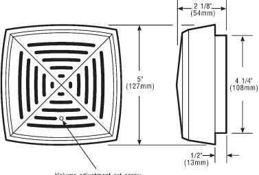
Volume adjustment set screw 1/16" (2mm) allen wrench supplied
